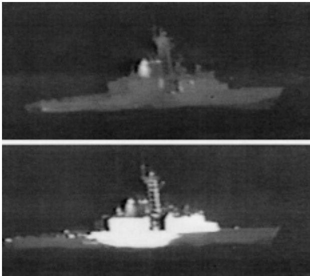
Figure 5 Solar Glint From Typical Navy Grey Paint
