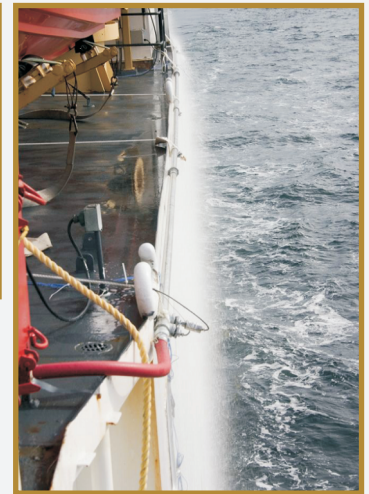
Left: MWIR measurement of ship with AHC on hull section (~ 10 km range); Middle: Fan nozzle; Right: Hull cooling on experimental ship.
