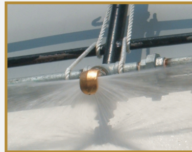
Left: MWIR measurement of ship with AHC on hull section (~ 10 km range); Middle: Fan nozzle; Right: Hull cooling on experimental ship.
