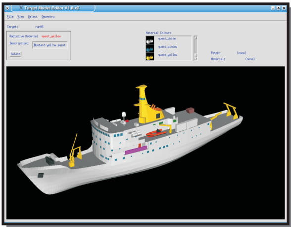
Top: User interface of ShipIR/NTCS; Bottom: Target Model Editor module of ShipIR/NTCS.
