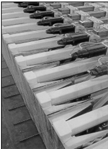
CEPYC Waveboards and Actuators
