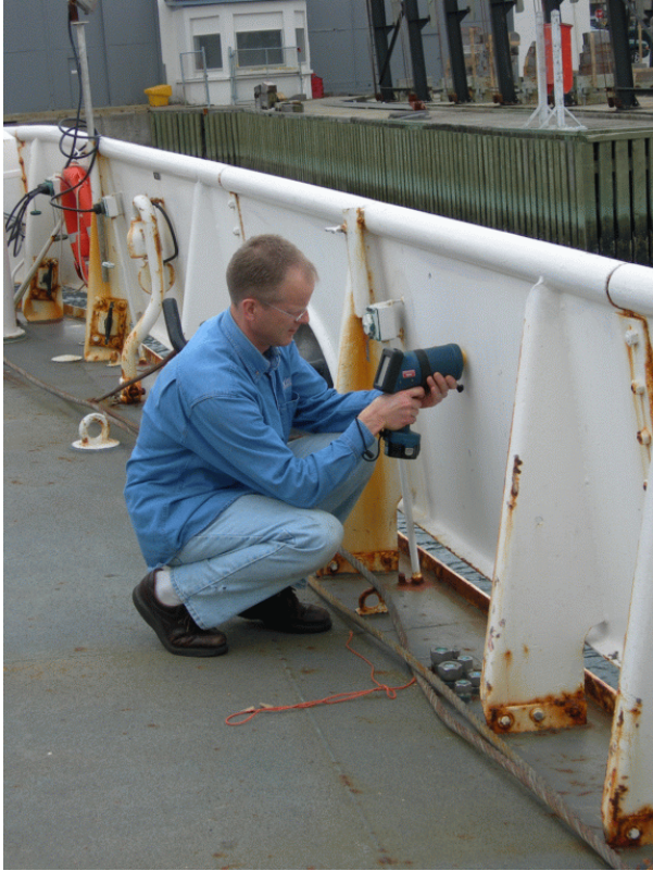
Figure 17: Direct sample using SOC-410.
