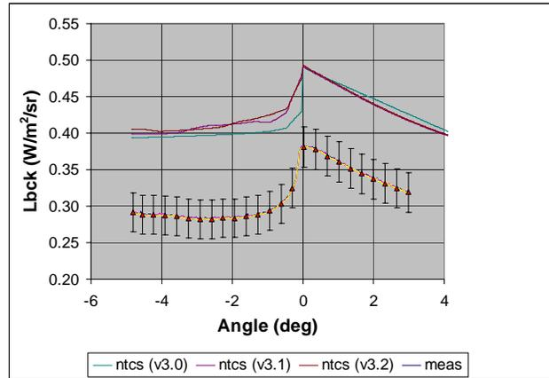
**Figure 8:** 3–5 $\mu\text{m}$  background radiance on clear day (Q276, run05) using a different versions and a standard atmosphere (mls).
