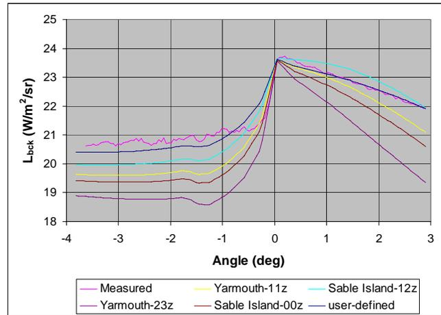
**Figure 6:** 8–12 $\mu$ m background radiance on clear summer day (Q262, run08) using different radiosondes.
