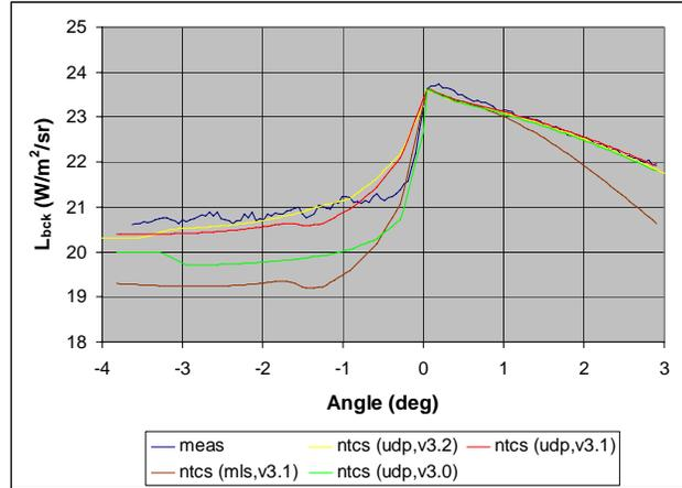
**Figure 7:** 8–12 $\mu\text{m}$  background radiance on clear day (Q262, run08) using different versions and a user-defined profile (udp).
